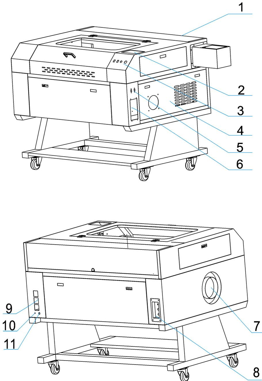
Note: 1·Back Cover (For laser Tube, refer to 3.1), 2·Control Panel, 3·Auxiliary Control Area
