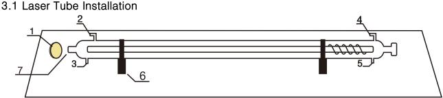
1. Mirror Holder 2. Water outlet 3Cathode- 4. Water in 5. Anode+ 6. Tube holder 7. Laser out
