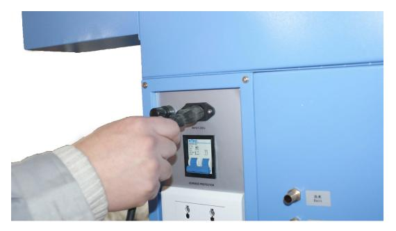
Connect the machine with the computer
