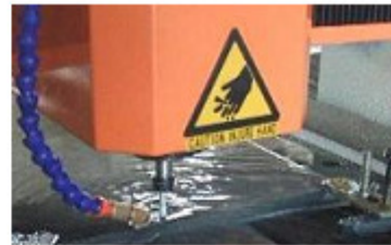
Water Cooling System
