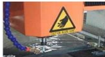
Water Cooling System
